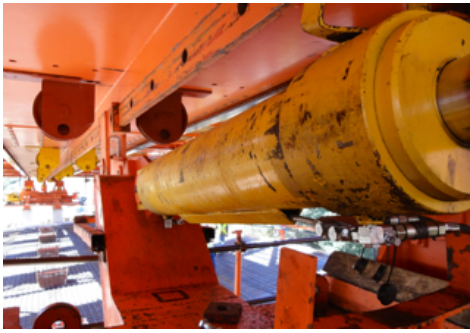
Detail of the launching cylinder
